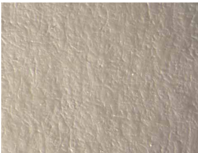
Paper coated with Duroblade-Silkoat (left) shows a finer, more even surface finish than the same paper coated using a conventional ceramic-tipped blade (both images magnified x25).
