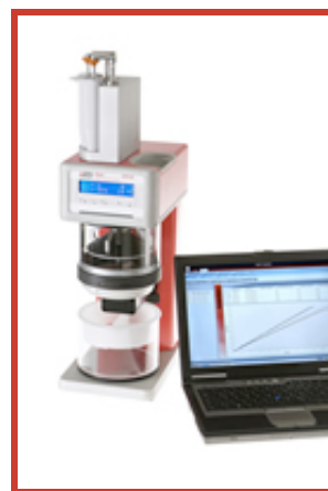
Figure 1: Mütek DFR-05 Drainage Freeness Retention
