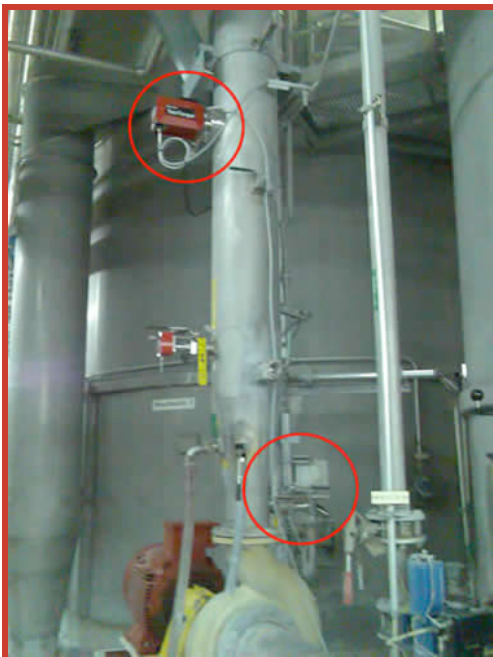
Figure 1: Installation of both sensors in the mill (MEK-3000 at the top, TCT-2302 at the bottom.)
