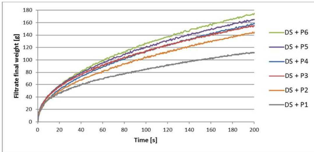
FIG. 3: DFR measurements of digested sludge after reaction with six different polyacrylamides (P1 to P6)
