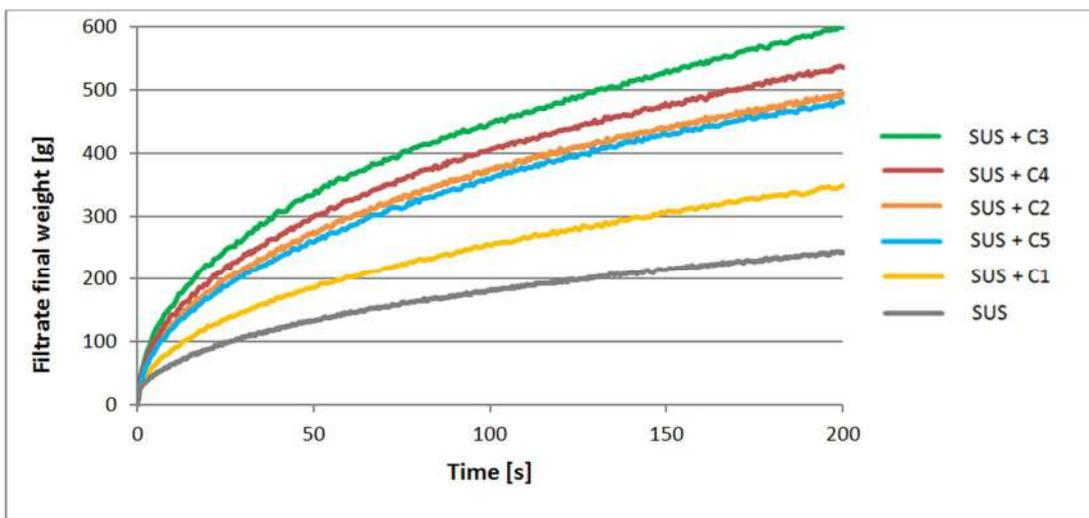
FIG. 4: DFR measurements of surplus sludge, untreated (SUS) and with different polymer concentrations (C1 to C5) added
