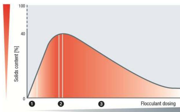
FIG. 1: Discharged dry solids vs. amount of polymeric flocculant: (1) Underconditioning, (2) Ideal conditioning and (3) Overconditioning
